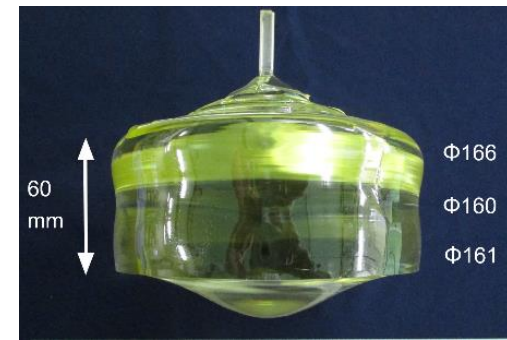
Production of lithium niobate (LN) crystal
