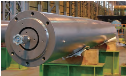
Steel pressure vessel for hydrogen storage
