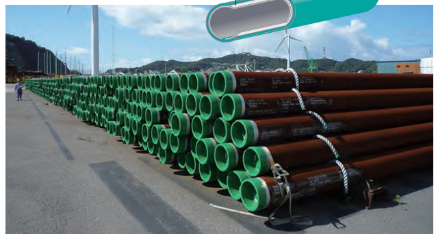
•Structure of clad steel pipe Inside: Stainless steel or high-alloy steel Outside: Carbon steel
