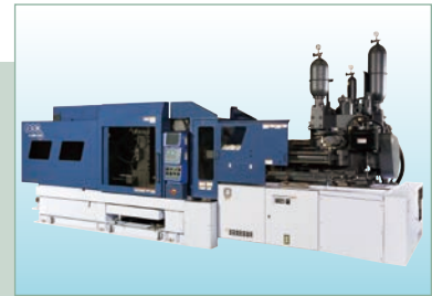
Magnesium Alloy Injection Molding Machine (280t)
