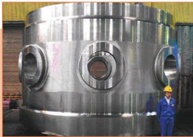
Shell Flange Used for Pressure Chamber for Nuclear Power Plant
